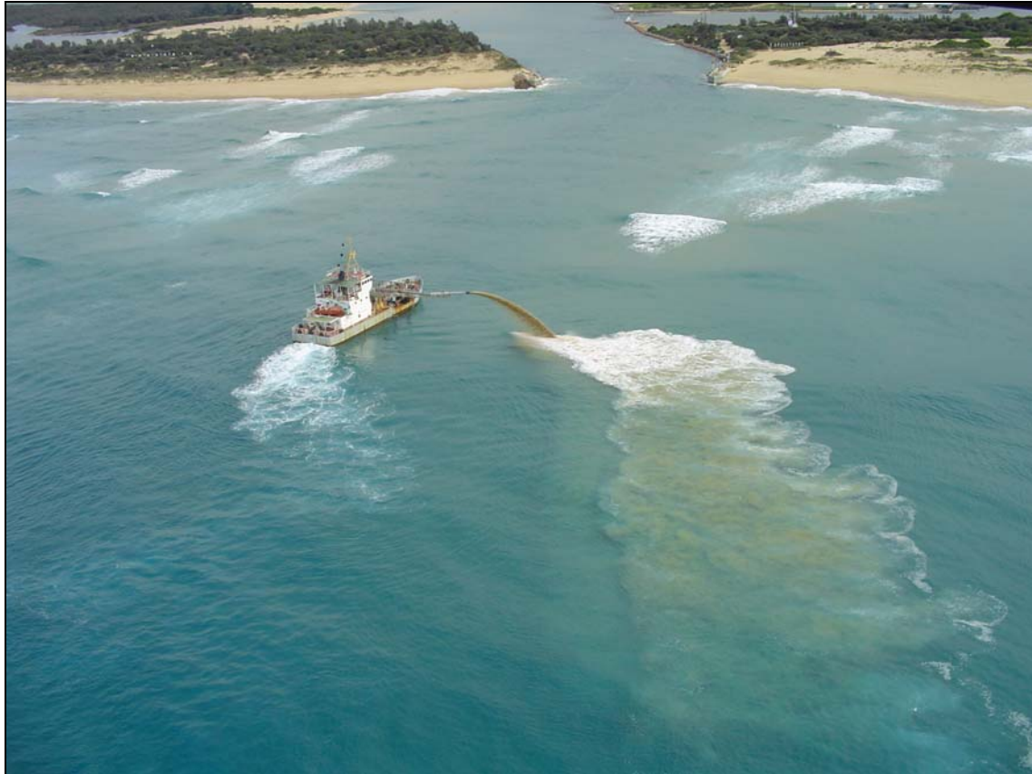
Fig. 6 The Gippsland Ports side-cast dredger April Hamer during dredging operations at the ebb-tide delta in Bass Strait on an ebb-tide. Source: Wheeler (2005)
